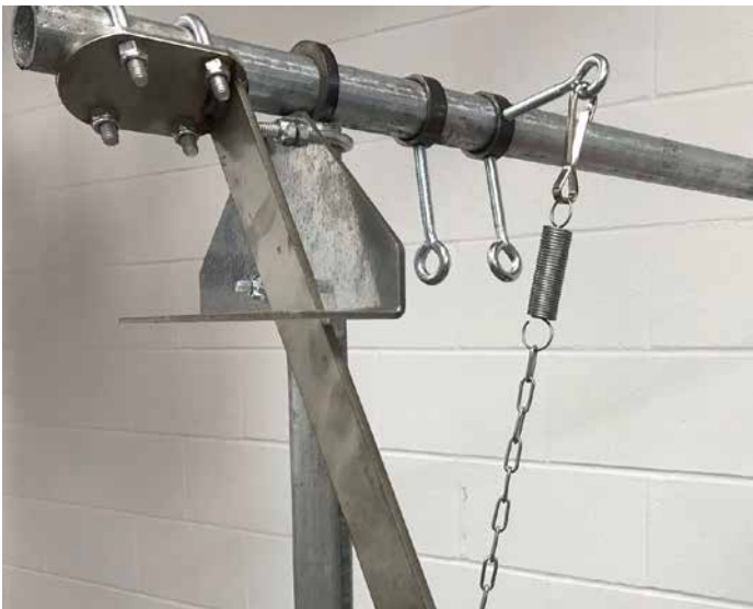
OPEN POSITION: Lever handle is positioned towards the chain in the lever bracket to re-engage locking tab.
