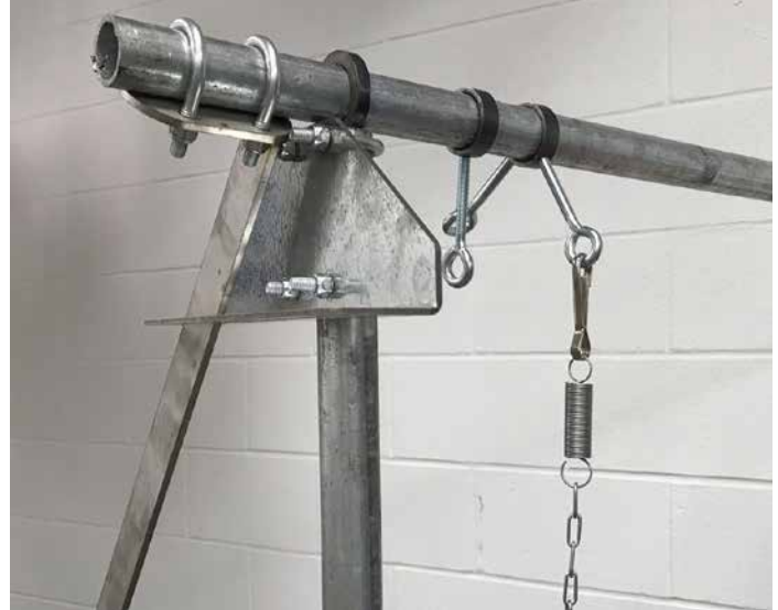
ROW LOCKING POSITION: Lever handle is positioned away from the chain in the lever bracket to lock a row of sows.
