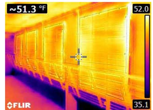
This FLIR photo was taken at the same finishing site in eastern Iowa 15 minutes after the PigTek Shutter Blank was installed on the 54-inch (1372-mm) fans. Note the reduction in cold air leakage and insulation provided on the fans as depicted by the uniform yellow/orange tones captured by the FLIR camera.
